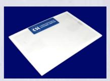
space for antenna mounting, such as display cabinet, smart-shelf and conveyor-belts etc. Thus, this antenna is the best choice for using in retail applications, production line, document control and any applications require thin form factor antenna.
